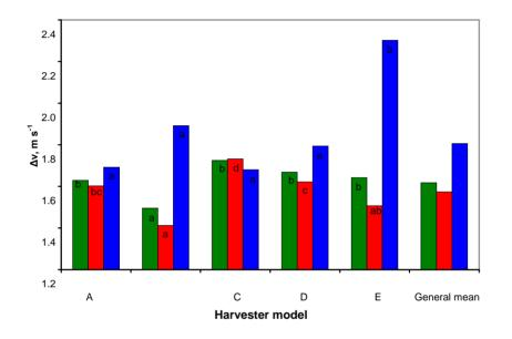
The velocity change  $-\Delta v$ - showed more variation (Figure 7). In zone 1, the lower values for  $\Delta v$  were registered in B and E. Therefore, the impacts on less absorbing surfaces occurred in these harvesters. D and A showed medium values for this variable and C reached the highest values. In zone 2, E showed significantly higher  $\Delta v$  impacts.
