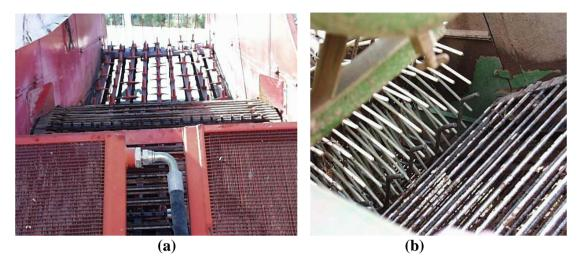
Figure 1. Harvester shaker systems: (a) belt shaker and (b) rotary shaker.
