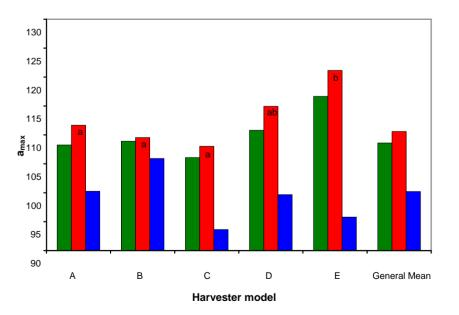
Figure 6 shows the impact intensity registered on each combine harvester and zone. Data distinguishes two groups in zone 1, with E having higher impact intensity compared to all other machines except D which is intermediate. In zone 2, there are no statistically significant differences between the five combine harvester models. There were no significant differences between the different combine models for harvester mean  $a_{max}$  variable.
