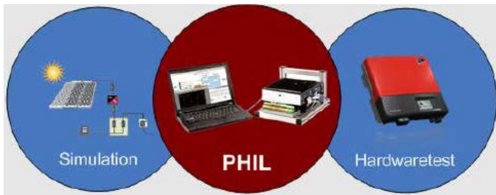
Fig. 3-5: (Power) Hardware-in-the-Loop technique [122]
