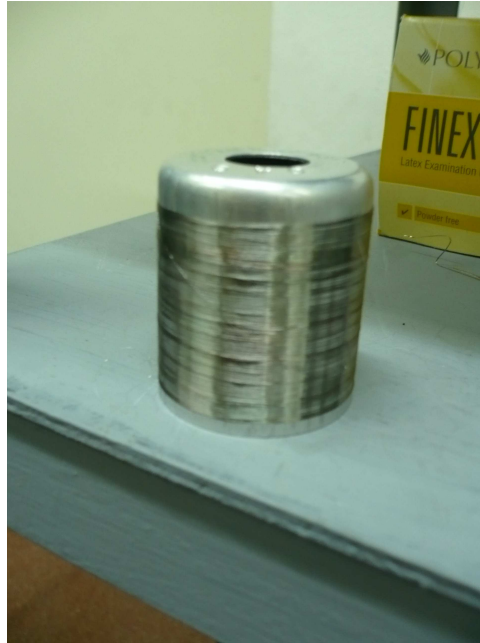
Figure 1.3 – Photograph of a single ferromagnetic wire forming a roll. (The photograph was taken during the fabrication of the wires at the Material Science Institute of Madrid (ICMM))
