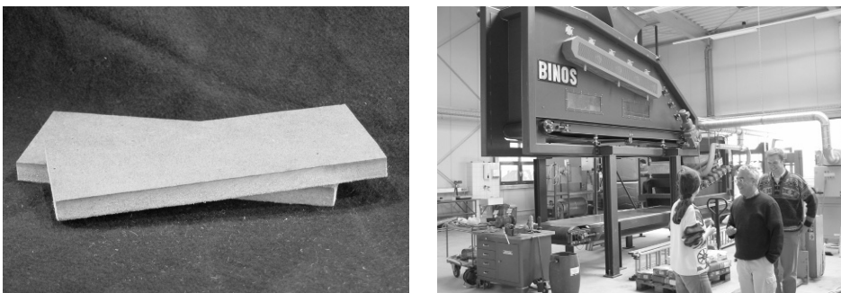
Figure 1. Medium-density fiber boards (MDF) of 1 cm thickness produced with a raw laccase extract from Pleurotus ostreatus (left) and the MDF-pilot plant at the Institute of Forest Botany (right). Details of the laccase-MDF-production process are found in Kharazipour et al. (1997).
