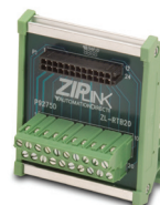
ZL-RTB20 20-pin feed-through connector module
