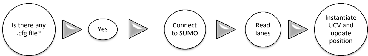
Figure 5: schematic representation of the first steps performed by CoAutoSim3D
