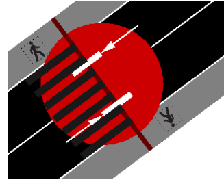
Figure 12: example of lane connections in netedit after edition
