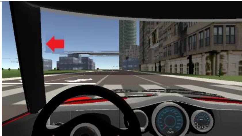
Figure 34: driver-centric perspective of a dangerous situation when the detection system is active
