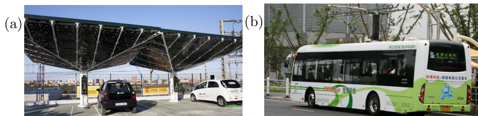
Figure 6.11: Transport applications of SCs: Electric car charging station in the foreground and railway track in the background. Lithium batteries and supercapacitors are used for the regenerative braking of railways and fast charging of electric vehicles [ADI]. Reproduced by kind permission of Adif (a) and Capabus charging its ESS based on supercapacitors. Reproduced from Wikipedia (b).
