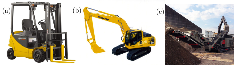
Figure 6.14: Industrial machines that use SCs. FB15HB-12 battery – SC hybrid forklift for Komatsu (a), PC200–8 Hybrid Excavator (b) and Rockster R1100DE Parallel Hybrid Crusher (c). Photos taken from the manufacturers websites.
