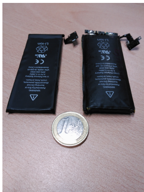
Figure 2.12: Fresh and swollen pouch cells used in an iPhone cellular.
