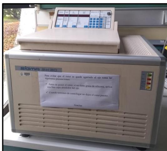
**Figura 3. Centrifuga Sigma 3K30.**
