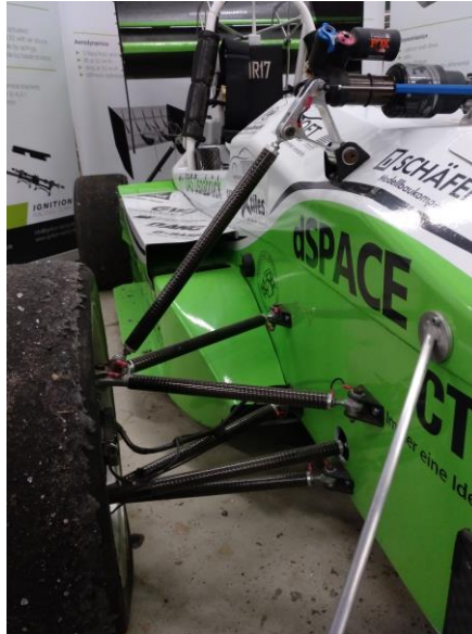
23 [Suspension of the 2016/2017 vehicle. The pushrod is the carbon rod positioned with approximately 45 degrees with respect to the ground]
