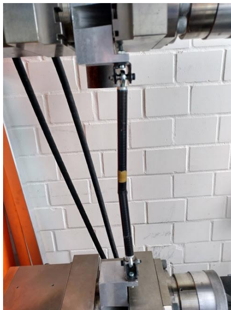
58 [Sample 16.3 breaking in the carbon tube]
