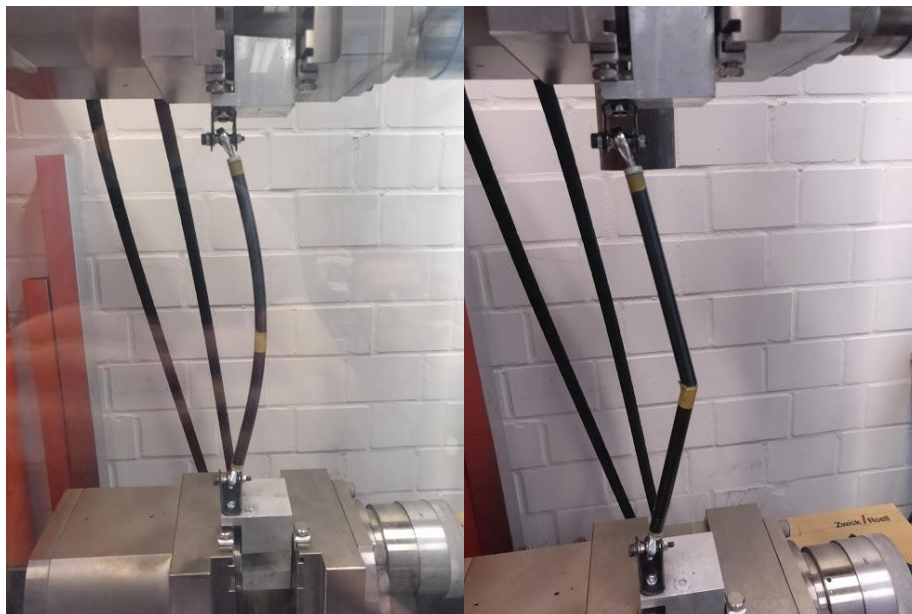
55 [Failure of the 12 mm carbon tube in the compression test]
