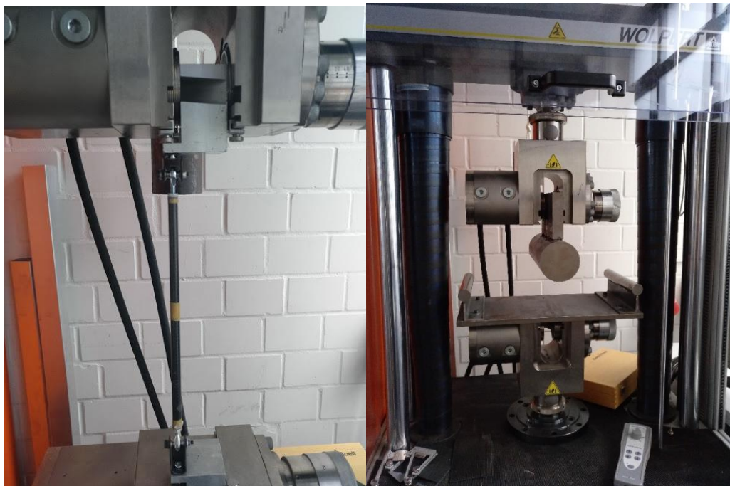
46 [Testing machine with both, tensile/compression and bending disposition]
