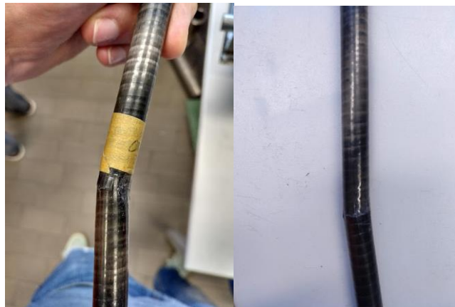
68 [Failure at bending of the carbon tubes]
