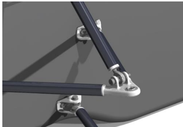
89 [Positioning of the union of the pushrod]
