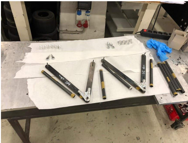
77 [A-Arm components ready to apply the resin]
