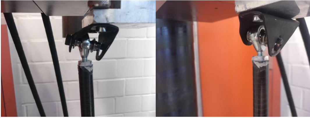
56 [Failure of the self- manufactured tool in the compression test]
