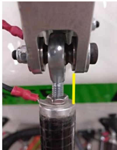
24 [Screwed condyle to the carbon tube. Screwing the condyle is possible to reduce the distance represented by the yellow stripe]
