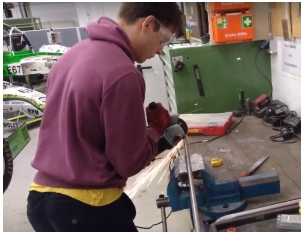
72 [Cutting a bar of alloyed steel of 24 mm diameter for the manufacturer ZF to manufacture the inserts of the carbon tube]
