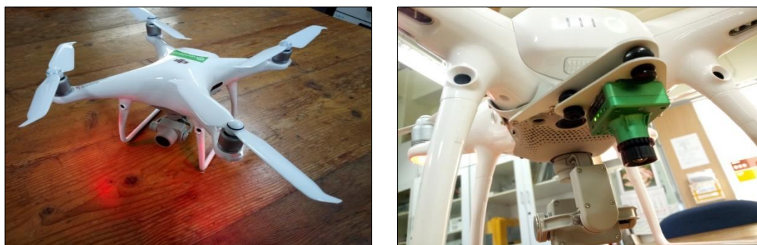
Figure 8 UAV montage. DJI Phantom 4 PRO v2.0 with a Sentera High resolution NDVI single sensor assembled (in green. Right picture) and the 4K RGB camera (in grey. Left picture).
