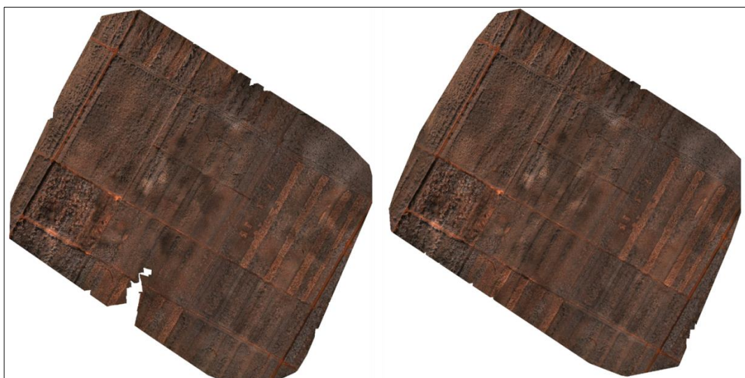
Figure 7 Real case of bad orientation problem. False color RED-NIR map. Bad orientation of images captured in a specific area produces "gaps" in the final orthomosaic (left), this issue can be corrected, depending on the level of miss-orientation, by a recalibration of the cameras (right). Notice that there still are zones of missing data in the boundaries which should be avoided by selecting a ROI.
