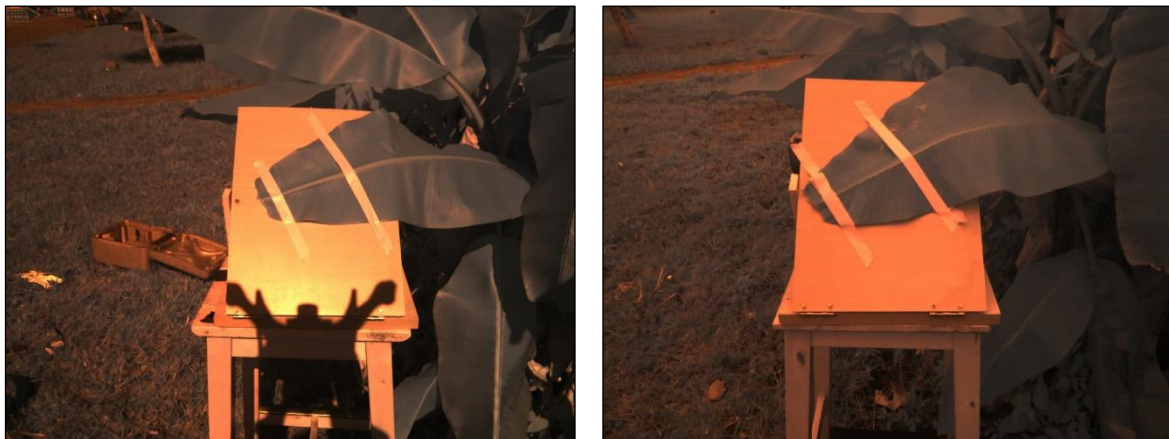
Figure 19 False color pictures (Red-NIR) employed for the overall performance and light dependency test. Picture capture the 20 th December (left) during “sunny” day and the 24 th December (right) under complete “cloudy” day.
