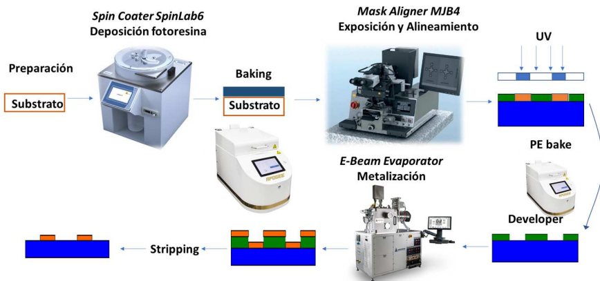
Figure A.1: Schematic of the photolithography procedure at the Public University of Navarra's facilities.
