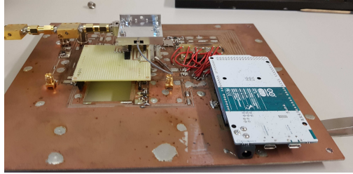
Figure 3.26: Y-Factor setup for fourth harmonic mixer characterization.
