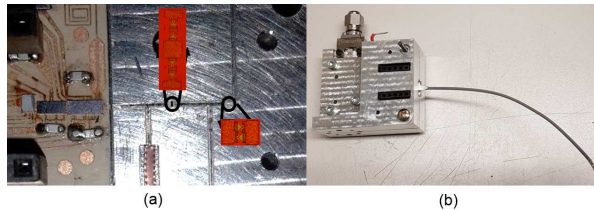
Figure 3.30: Photograph of the subharmonic mixer mounted in the metallic housing block: (a) MMIC source and doubler/subharmonic mixer with inset of the UMS diodes. (b) Enclosed housing metallic block.
