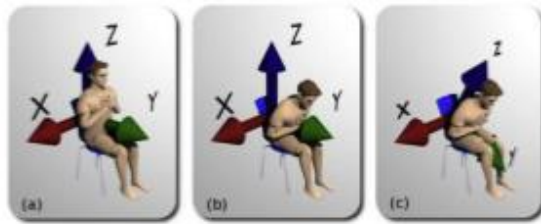
Fig. A1. Changes in global and IU's local Cartesian reference axes when the subject is trying to stand up at the beginning of the 30-s CST. The first figure, (a), depicts the initial position; global and local reference axes coincide. When the subject changes position, the global axis remains unchanged (b) whereas the IU's local reference axis rotates with the physical device (c).
