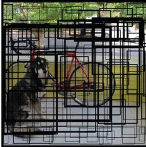
Figure 13: Example of the bounding boxes predicted in each cell; the high confidence boxes are drawn fatter.
