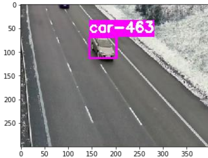
Figure 53: Reduced frame to the right lanes with shape (400,300)
