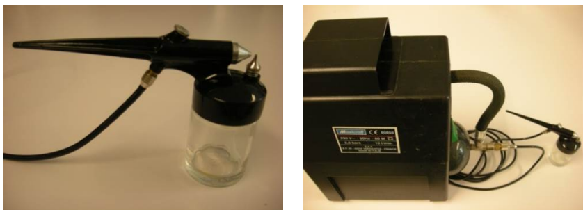
Figure M.M.4. Detail of the aerograph used for the treatment application (A) and the aerograph connected to a compressor (B).
