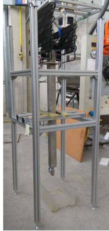
Figure 3: GTEG with phase change heat exchangers developed and studied by Catalan et. al [20].
