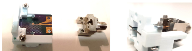
Fig. 15: Picture of the mixer before the IF end-launcher connector assembly on the left and final assembled device on the right.
