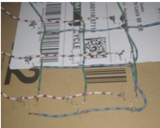
Figure 9 Wiring of the sensor matrix
