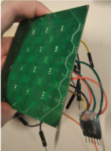
Figure 39 Side view of the 2 stacked and wired PCBs
