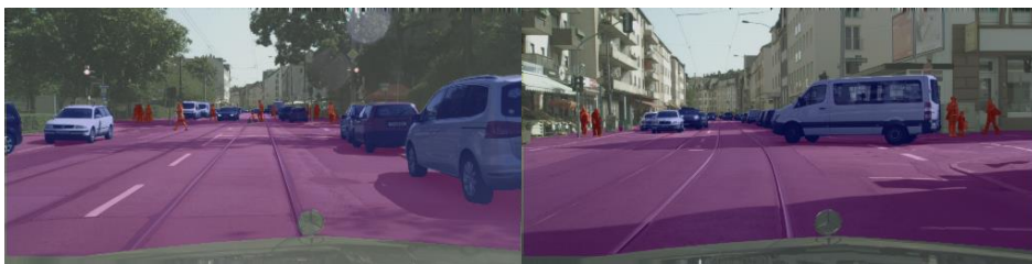
Image 9. Example of two training images with their corresponding masks overlapped (each color represents a different class)
