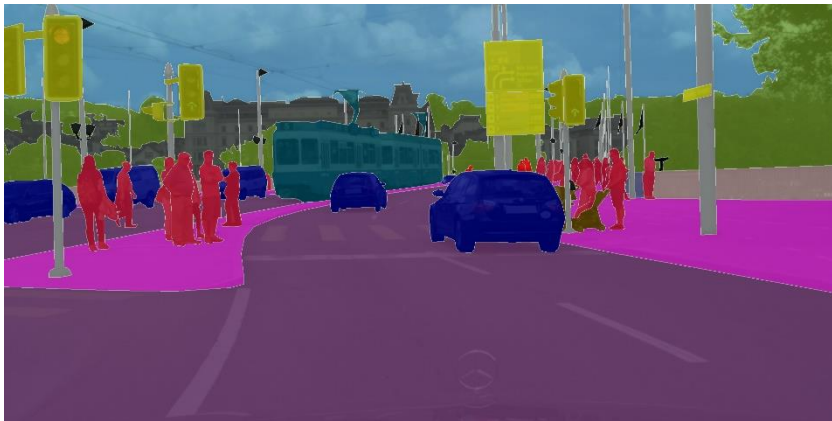
Image 10. Example of annotated image taken in Zurich (Overlaid colors correspond to the 30 semantic classes) [16]
