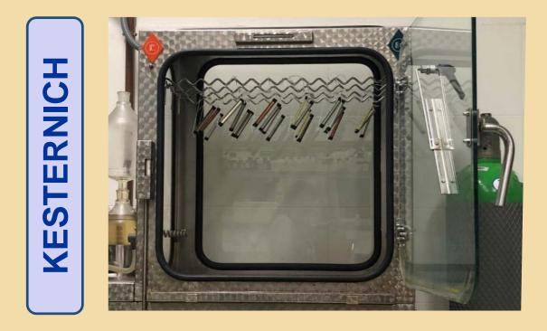
0.2 L SO<sub>2</sub>(g) and 100% humidity, 10 cycles. After Kesternich test, weight loss, MO, SEM and XRD analyses have been performed.
