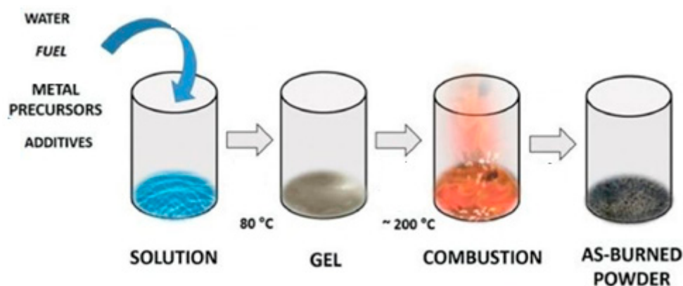
Figure 20. Schematic showing the steps in a typical combustion process (Adapted from [60]).
