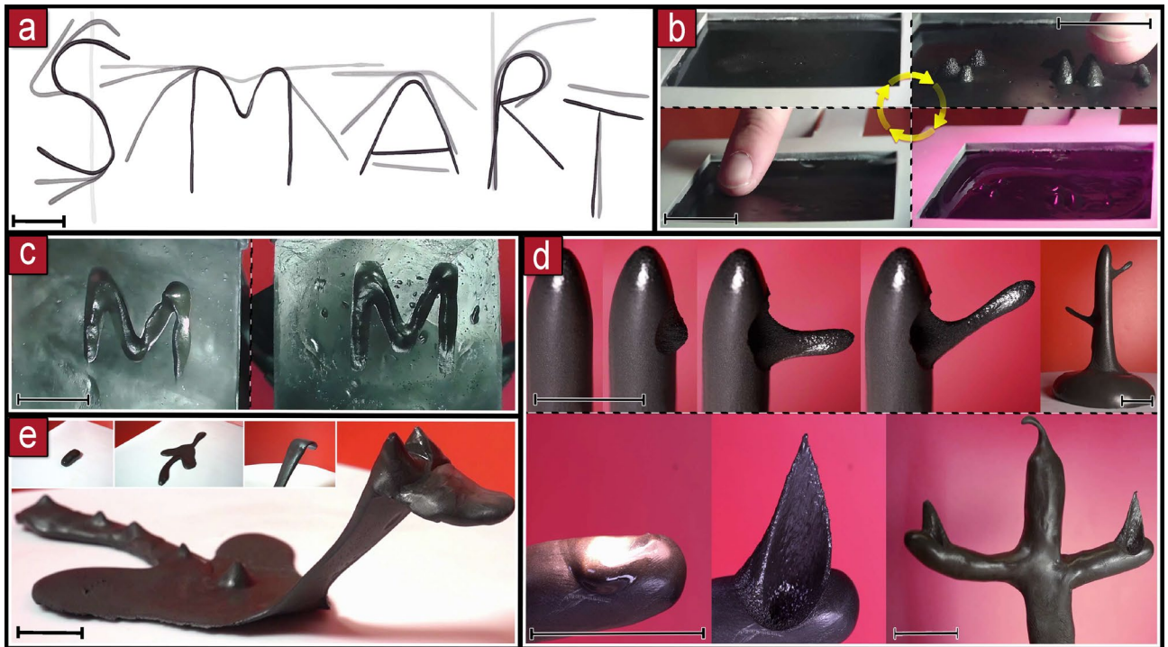
Figure 4. Complex manipulation. (a) Forming letters with 1D filament. (b) Reversible Braille patterns on a sheet. (c) Embossed letter M on a sheet. (d) Branching. (e) Sculpting in 3D. Scale bars are 3 cm.
