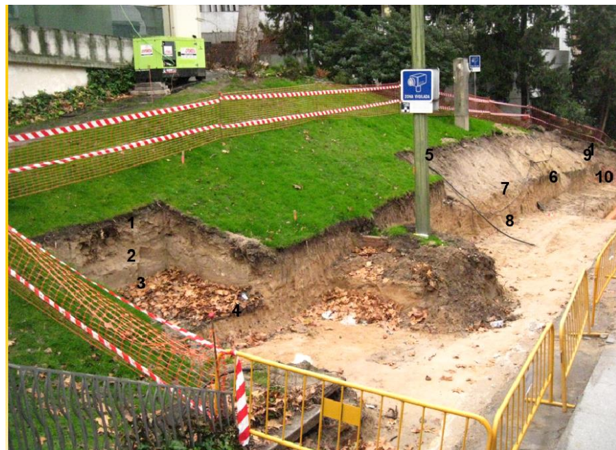
Figure 2. Garden soil profile formed of an artificial mixture of several internal and external artifacts. Samples 1 to 10 correspond to the analyzed soil samples. Sample 2 depicts the bricks, rubble and debris substrate mediums embedded in horizon Bwp; Samples 4, 6, 7 correspond to humic topsoil above mixtures of arkose material, ash and bricks, and probably sludge; Samples 9, 10 are horizons on slightly sealing-consolidated and not segregated substrate, partly crushed and massive. At the bottom, a sewer ditch filled with sand and other cement materials.
