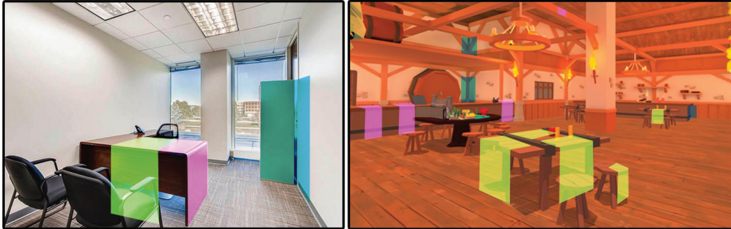
Figure 5.13: Examples of a few surfaces and shapes scanned from a regular office being mapped into different locations inside a fantasy VR tavern. Depending on the user's real-life location, it can move and interact with different virtual elements reusing the same surfaces. Note that much more shapes could be reutilised between worlds.
