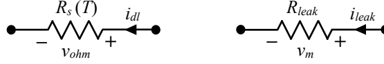
Fig. 4. Equivalent circuit for the ohmic losses in an SC cell. Ion and electron conduction losses ( R_s , left) and membrane losses resulting from self-discharge ( R_{leak} , right).
