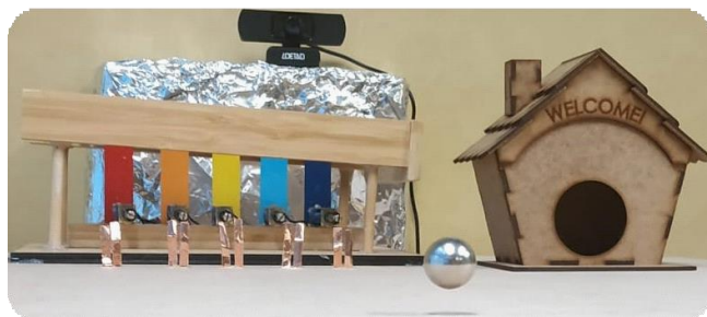
Figure 1: The LevPet system. Sr. Boliche is levitating above its playground. At the left, the xylophone and the webcam to recognize the user. At the right, the house where the pet can take cover or go to rest.
