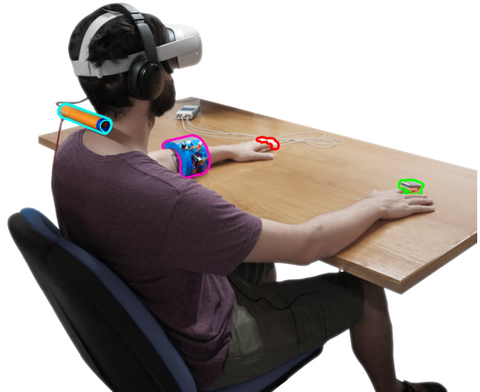
Fig. 19. A user conducting the pilot experience study. Wearing VR glasses (Quest 2) and noise-canceling headphones. The electrode (cyan) was above the nape at 3.5 cm. On the non-dominant hand, the galvanic skin response was measured with grounding on the ring and sensing on the index and heart fingers (red); a wearable close-zoom camera with illumination recorded the forearm, checking for piloerection (fuchsia). On the dominant hand, the heart-rate was measured with a pulse oximeter (green).
