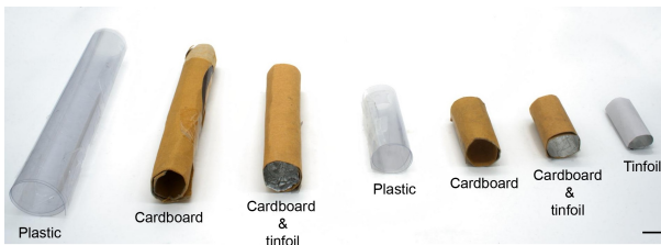
Fig. 9. Tested electrodes (left to right): plastic (20.3 cm long, 3.3 cm diameter), cardboard (17.7 cm long, 2.5 cm diameter), cardboard with tinfoil (13 cm long, 3 cm diameter), plastic (8 cm long, 3.1 cm diameter), cardboard (5.4 cm long, 2.5 cm diameter), cardboard with tinfoil (4.4 cm long, 2.5 cm diameter) and tinfoil (4.8 cm long, 2 cm diameter). Scale bar is 1 cm.
