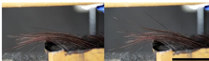
Fig. 7. Fake hairy skin made of silicone and graphite with fake hairs grafted, the cardboard electrode is above the hairs. Left) without electrostatic piloerection. Right) with electrostatic piloerection activated. Scale bar is 3 cm.
