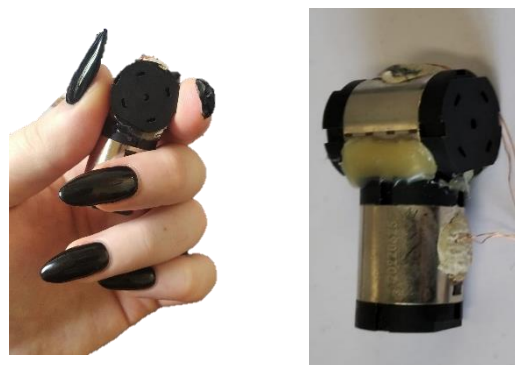
Fig. 14 2DoF device on the right, and its holding position, thumb contacting both actuators, index and middle fingers on different actuators.
