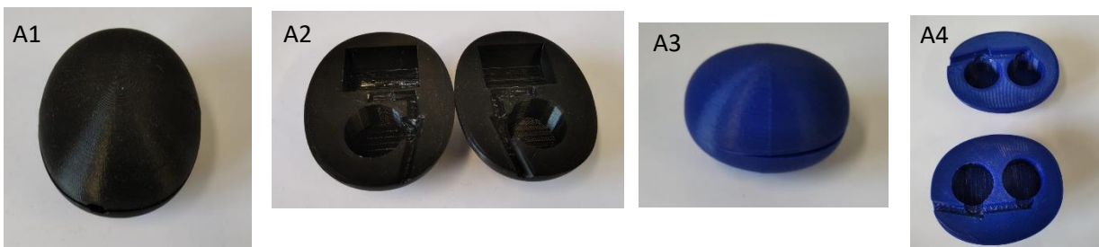
Fig. 16 Different casings for the actuators. A1, A2 was intended for a 2DoF device, while A3, A4 was intended to increase the strength of the sensation by using 2 actuators.
