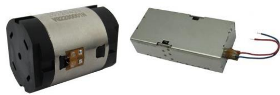
Fig. 1 Voice coil actuator and LRA [12]-[13]
