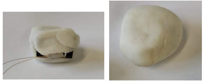
Fig. 15 Actuator partially encased in plastic (left), and fully encased (right)
