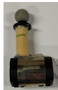
Fig. 23 GuidingHaptics device with reflective marker on top of a cardboard tube.
