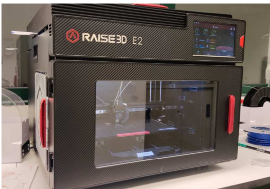
Fig. 3. RAISE3D E2 dual extruder FDM printer used for prototype fabrication.
