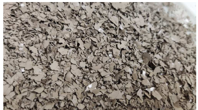
Fig. 1. Mixture of ABS pellets with silver-based micro and nanoparticles.
