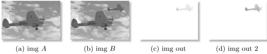
Fig. 8. In Fig. 8a we see the image (named A ) of a flying plane. In Fig. 8b we see a modified version of Fig. 8a (named B ). Fig. 8c comes from applying Algorithm 1 with input images A and B , and choosing as restricted equivalence function the one presented in Example 4.2, namely F(x, y) = 1 - |x - y| if |x - y| < \frac{1}{2} ; F(x, y) = \frac{1}{3}(1 - |x - y|) otherwise. Finally, Fig. 8d is the result of applying Algorithm 1 with input images A and B , but now choosing as REF the classical F(x, y) = 1 - |x - y| ; x, y \in [0, 1] .
