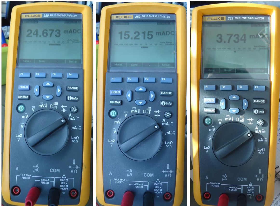
(c) Current consumed by the Lipmouse in the sleep mode and the BT switched off
