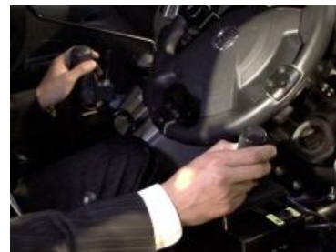
(g) Steering wheel adapted with joystick
