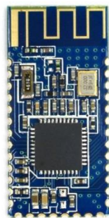
(a) HM-10 BLE 4.0 module (Source: modified from [25])
