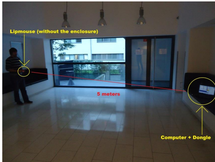
Figure 4.5: Test of the indoor coverage
