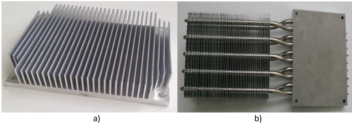
Figure 4. Heat exchangers on the cold side, a) finned dissipator, b) heat pipe.
