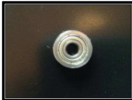
Figure 9 : Bearing . External diameter 12mm. Internal diameter 4mm. Widht 4mm.
