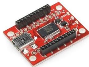
Figura 2.25. Xbee Explorer USB. [I19]
