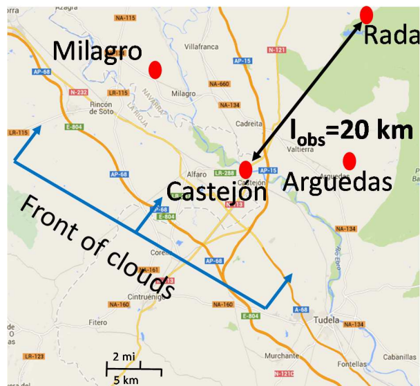
Figure 5.16: Calculation of \tau_{obs} for the PV fleet formed by Arguedas, Castejón Milagro and Rada ( N = 4 ) during the fluctuation on 16 th April 2013.
