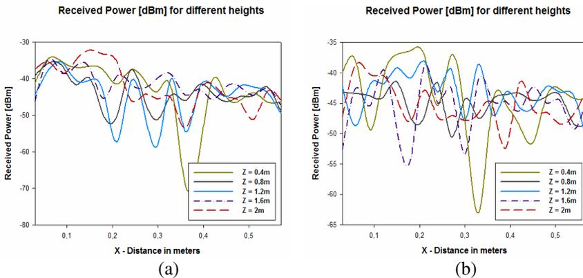
**Figure 10.** Estimation of received power for different heights within the simulation scenario. (a)  $f = 2$  GHz, (b)  $f = 2.4$  GHz. Reproduced courtesy of The Electromagnetics Academy
