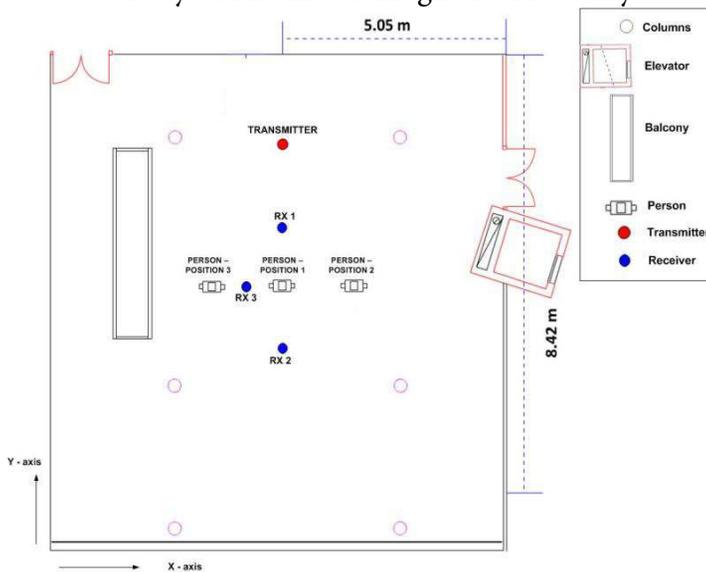
**Figure 11.** Scenario considered for the measurements. Reproduced courtesy of The Electromagnetics Academy
