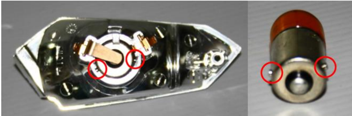
Figure 27: Bulb fitment Poka-Yoke
