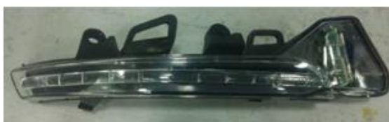
Figure 55: Fiat Linea Mirror blinker
