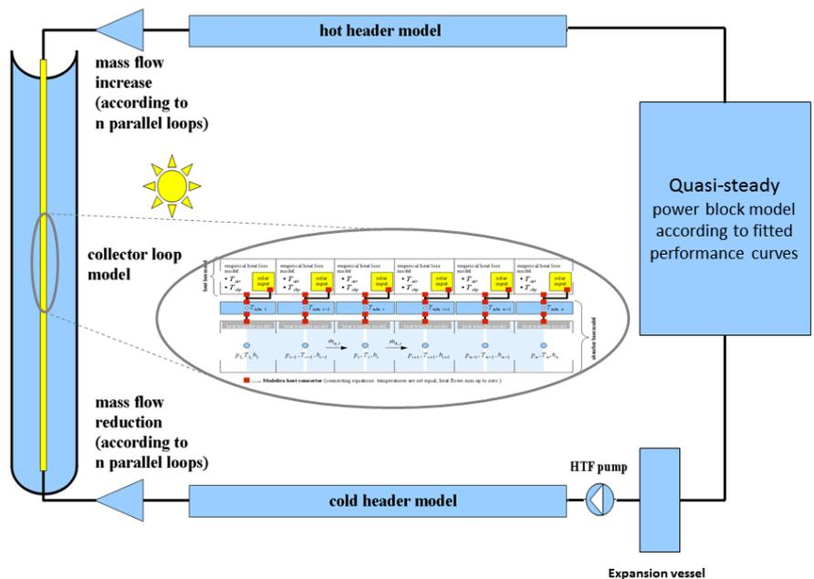
Figure 2. Scheme of the main parts of the parabolic trough plant model.
