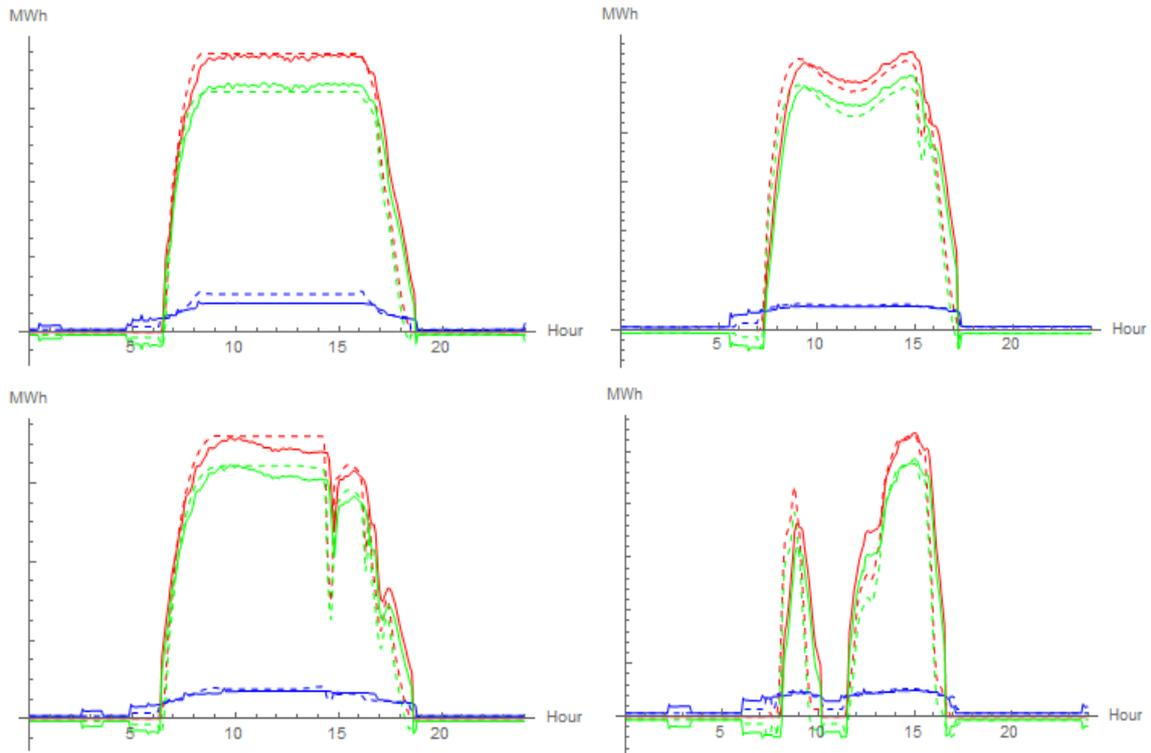
Figure 3. Comparison of the estimated (dashed) and measured (solid) for the gross power (red), net power (green) and auxiliary power (blue,) for a summer sunny day (top, left), an autumn sunny day (top, right), a summer sunny day with punctual clouds (bottom, left) and an overcast day (bottom, right).
