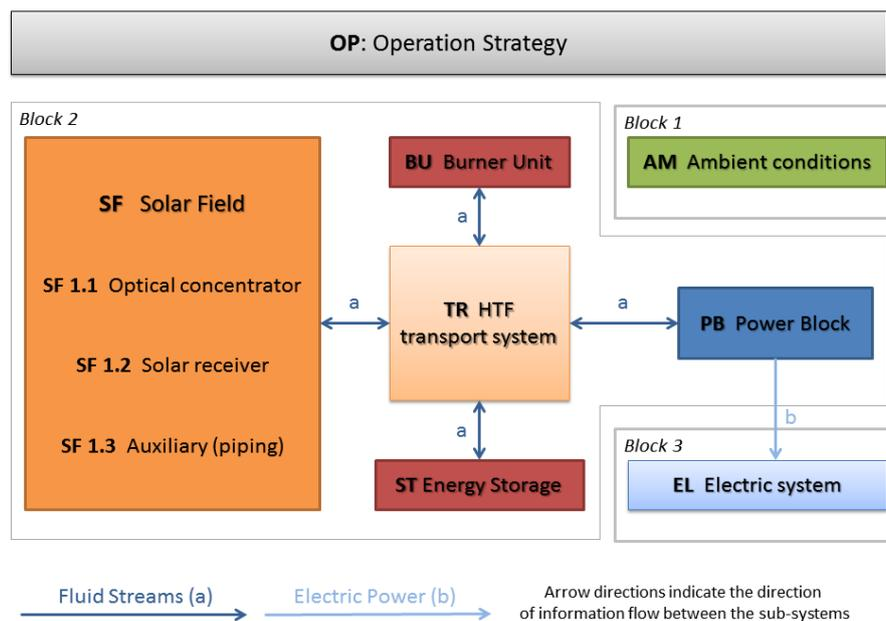
Figure 1. Scheme of the main parts of the CSP plant model according to the document [2].
