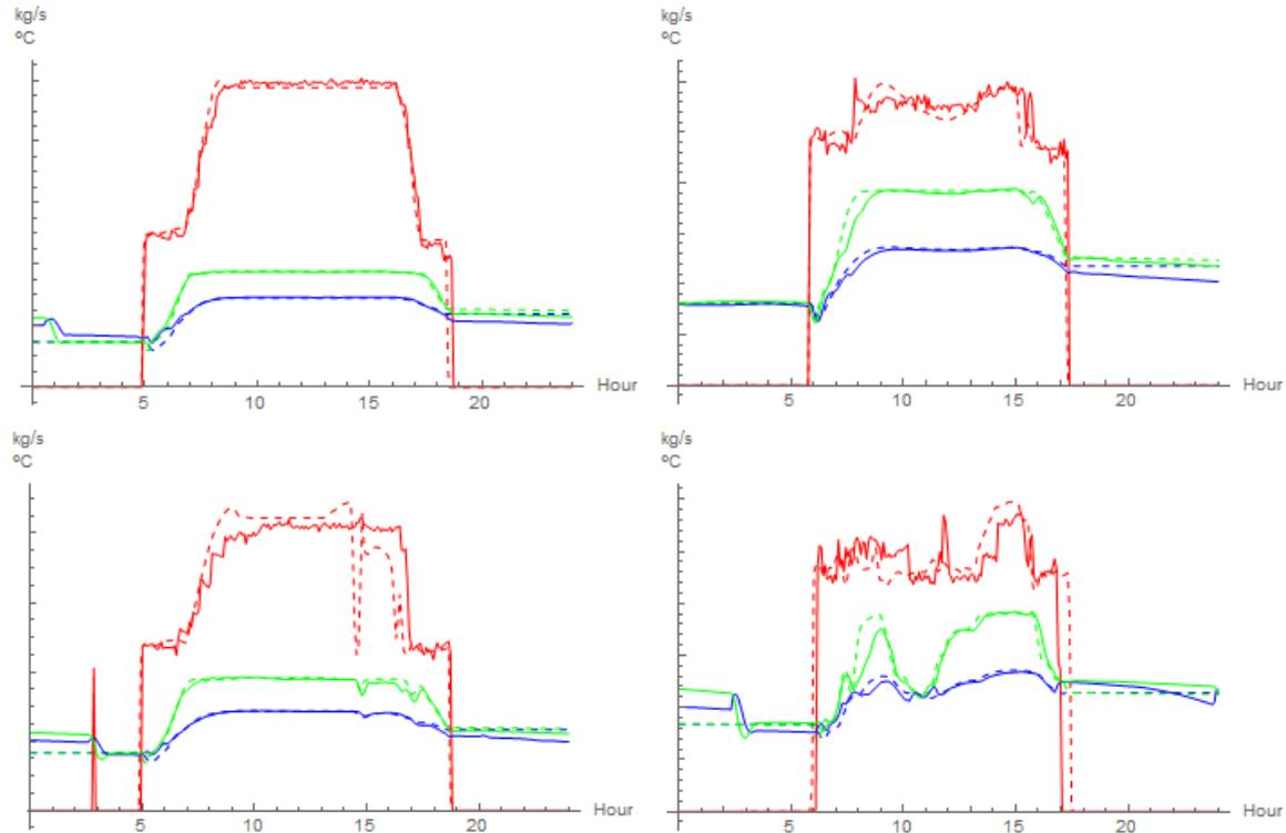
Figure 5. Comparison of the estimated (dashed) and measured (solid) solar field mass flow (red), outlet temperature (green) and solar field inlet temperature (blue), for a summer sunny day (top, left), an autumn sunny day (top, right), a summer sunny day with punctual clouds (bottom, left) and an overcast day (bottom, right).
