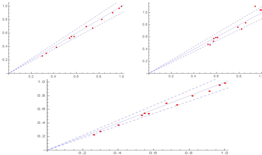
Figure 4. Comparison between the estimation and the measured data for all the days of the gross energy (top left), the auxiliary energy (top right) and the net energy (bottom).
