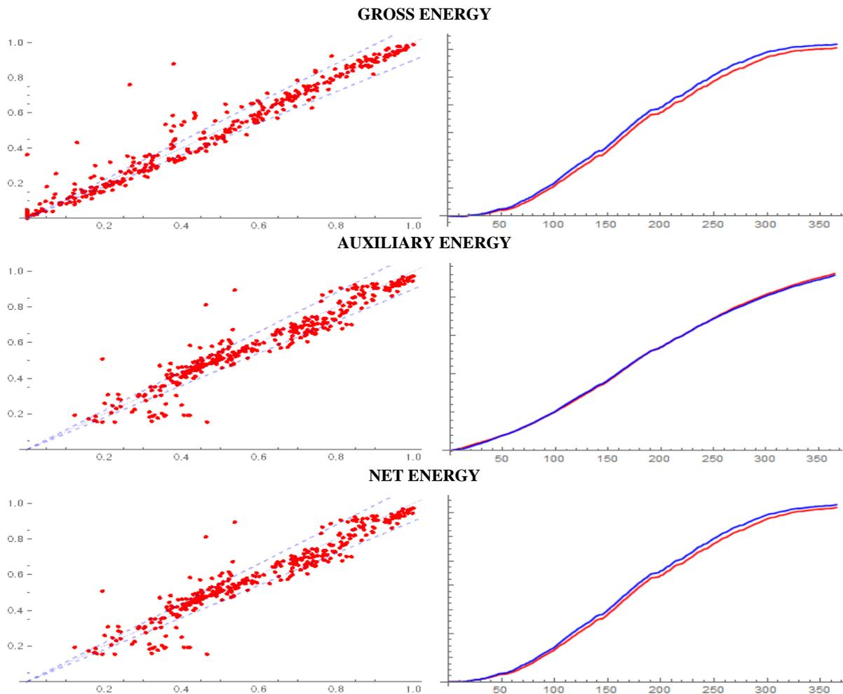
Figure 7. Comparison between the estimation and the measured data for all the year's days of the gross energy (top left), auxiliary energy (middle left), net energy (bottom left) and accumulative plot along one year, according to the software (blue line) and to measured data (red line) of the gross energy (top right), auxiliary energy (middle right) and net energy (bottom right).
