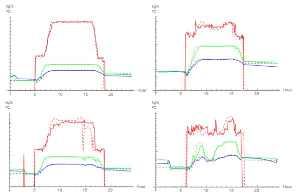
Figure 5. Comparison of the estimated (dashed) and measured (solid) solar field mass flow (red), outlet temperature (green) and solar field inlet temperature (blue), for a summer sunny day (top, left), an autumn sunny day (top, right), a summer sunny day with punctual clouds (bottom, left) and an overcast day (bottom, right).
