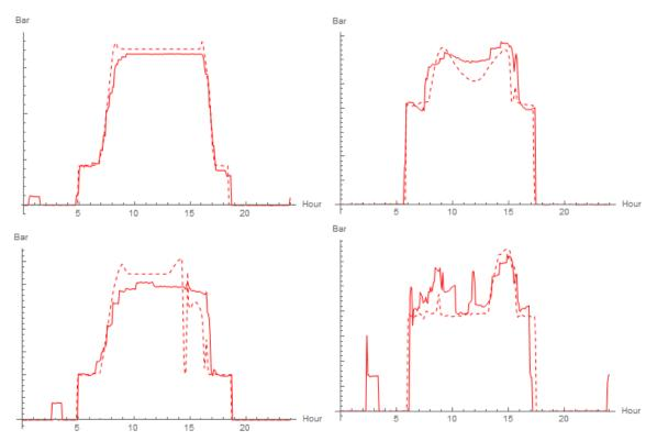
Figure 6. Comparison of the estimated (dashed) and measured (solid) solar field outlet pressure drop, for a summer sunny day (top, left), an autumn sunny day (top, right), a summer sunny day with punctual clouds (bottom, left) and an overcast day (bottom, right).
