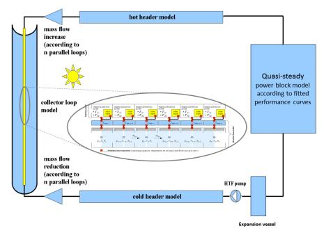
Figure 2. Scheme of the main parts of the parabolic trough plant model.
