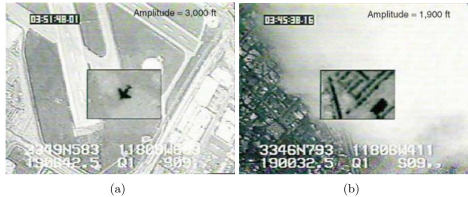
Figure 1.3 – Examples of reconnaissance and surveillance applications of PMMW imaging: Detection of a) an aeroplane C-17 and b) roadways and buildings through clouds [1].
