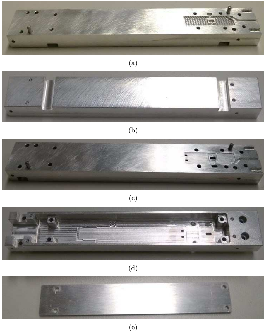
Figure 6.1 – Photographs of the manufactured aluminium packaging block: a) interior and b) exterior view of the top block of the packaging; c) interior and d) exterior view of the bottom block of the packaging and e) the cover.
