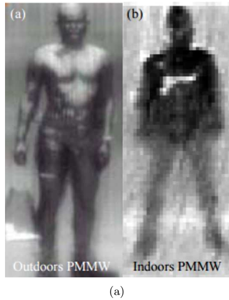
Figure 1.4 – Example of defence and security applications of PMMW imaging related to the detection of a gun at 94 GHz: a) Outdoors PMMW image of a man carrying a gun in a bag [25] and b) indoors PMMW image of a man with a gun concealed under clothing [26].
