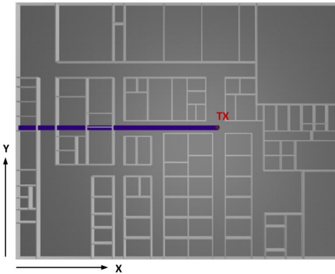
Figure 4.36. Top view of the full schematic scenario with the location of the transmitter and the radial line for comparison.
