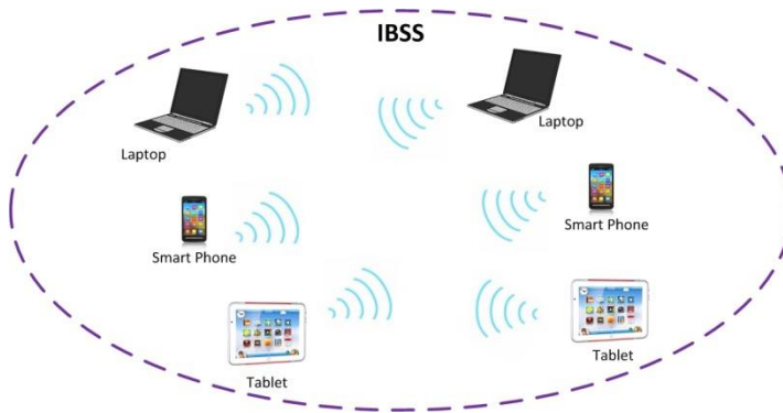
Figure 2.5. Ad hoc IEEE 802.11 network forming an Independent BSS.
