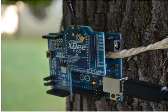
Figure 6.45. The ZigBee mote used for wireless communications in the vegetation environment.
