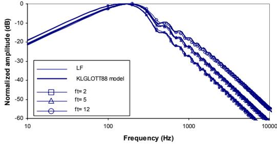
Fig. 7.a. LF and KLGLOTT88 spectra for different  $f_i$ .  $O_q = 0,4$
