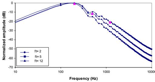
Fig. 2.a Spectral effect of  $f_t$ .  $O_q = 0,4$ .  $F_o = 100\text{Hz}$
