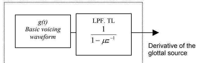
Fig. 1. Block diagram of the KLGLOTT88 model
