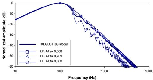
Fig. 8 Asymmetry coefficient in the LF model.  $O_q = 0,5$ ,  $f_i = 5$ .
