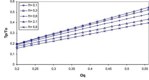
Looking at Fig. 4, a linear relationship between  $T_p/T_o$  and  $O_q$  is apparent, a thus it can be modeled as:
