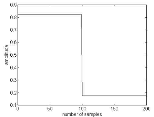
**Fig. 2.** Interpolation time domain window  $w_{SIDFT}$  for the *SIDFT* spectrum for  $a = 0.65$  and  $N = 100$
