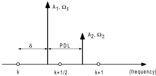
From Fig.4 it can be seen that the *SIDFT* is more effective when the magnitude difference is smaller. For larger magnitude difference, the discrimination process is corrupted by the "short term" leakage effect.
