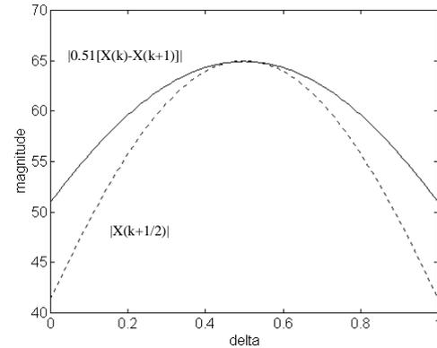
**Fig. 3.** A single peak interpretation: dotted line - *SIDFT* spectrum; continuous line - linear combination spectrum
