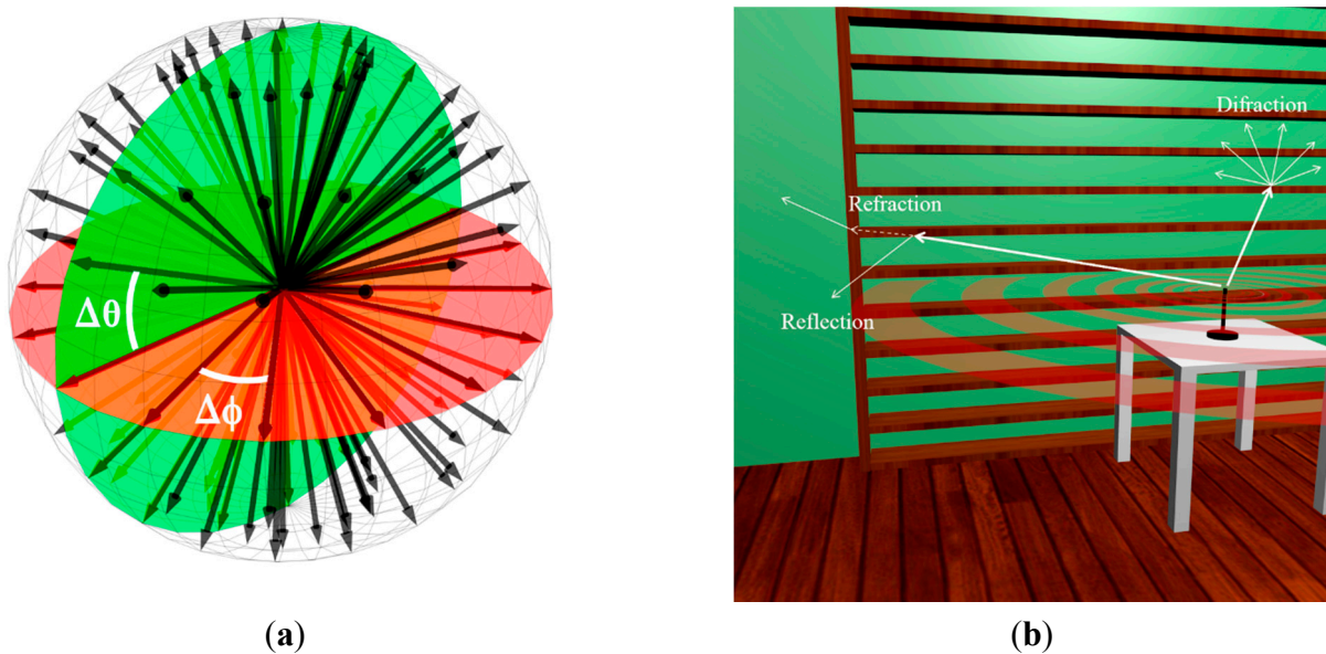
Figure 10. Principle of operation of the in-house developed 3D ray launching code, (a) angular resolution of launched rays; (b) electromagnetic phenomena within the scenario.
