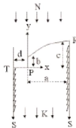
**Fig. 1a.** Flow field to be rectangular ditch without water and a permeable vertical wall with seepage (After v. Deemter).
