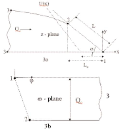
Fig. 3. Flow to a straight seepage surface. (a) The complex  $z$ -plane configuration, and (b) the complex potential-stream function representation.
