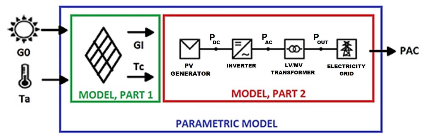
A parametric modeling requires precise and detailed information about the characteristics and behavior of each relevant component of the PV plant. This information is not always available so some simplifications and assumptions are needed, with the subsequent uncertainty in the output of these models.
