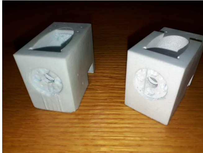
Fig. 71: Front view of the pieces made with SLA.
