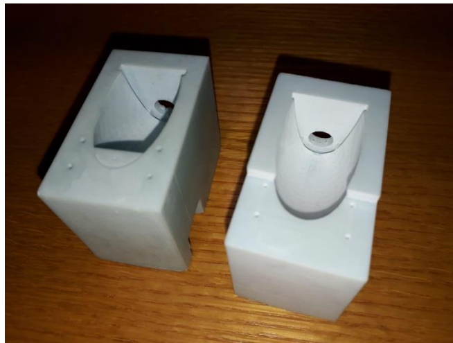
Fig. 72: Back view of the pieces made with SLA.
