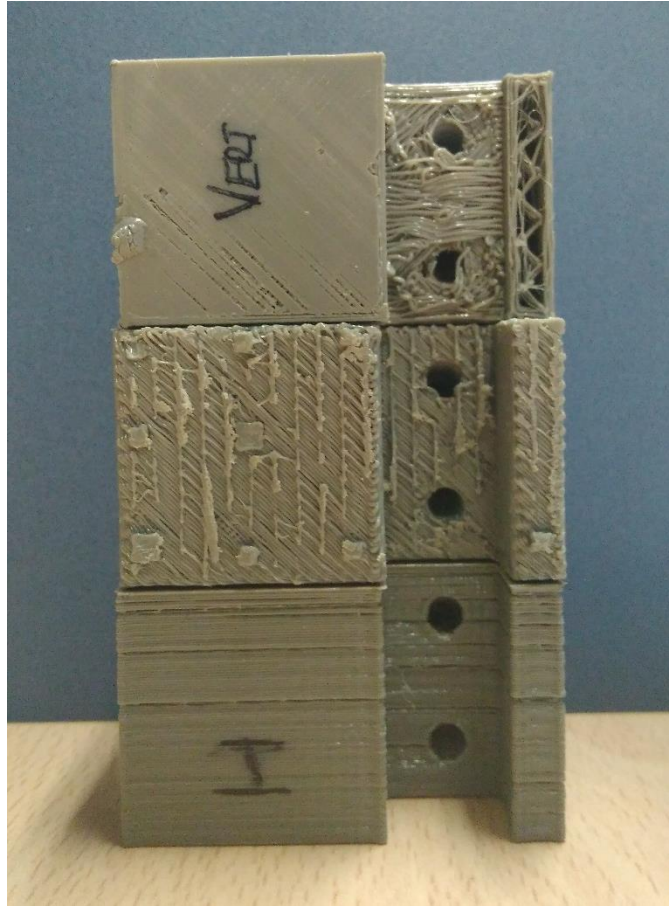
Fig. 70: Bottom view of the pieces made with FFF (Vertical / Rotated / Horizontal).
