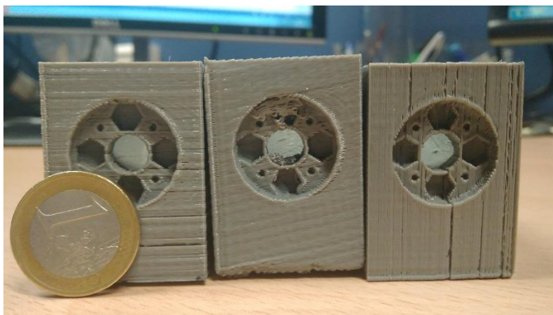
Fig. 69: Front view of the pieces made with FFF (Vertical / Rotated / Horizontal).
