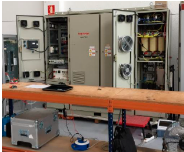
Figure 5.15: Test bench used for the validation of the proposed modulation strategies.
