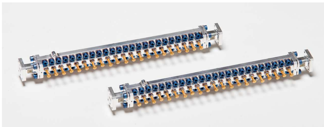
Figure 7.1: Q-band inductive-iris BPFs courtesy of Thales Alenia Space - Spain.
