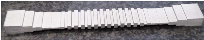
Figure C.2: Photograph of the mandrel of the corrugated E-plane low-pass filter.
