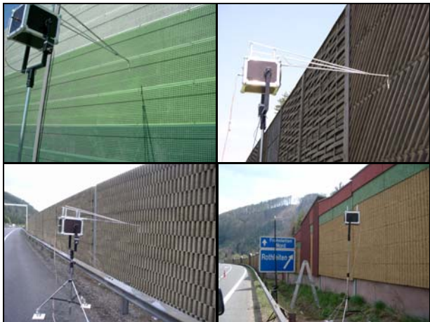
Fig.3 Test equipment during the measurements on the most common Austrian noise barriers (made of aluminums, timber and cement-bound wood chipping).
