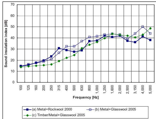
Fig. 13—Sound insulation index measured in situ in front of three types of cassettes: (a) full metal filled with rock wool, measured in the year 2000; (b) full metal filled with glass wool, measured in the year 2005; (c) mixed timber/metal filled with glass wool, measured in the year 2005.
