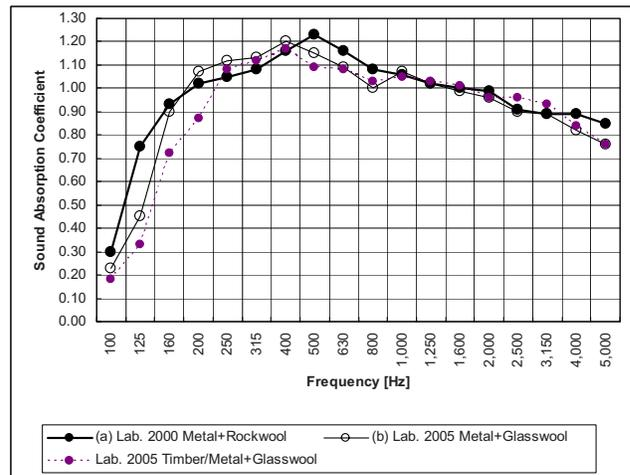
Fig. 8—Sound absorption coefficients measured in the laboratory. (a) metallic cassettes filled with rock wool, measured in 2000; (b) metallic cassettes filled with glass wool, measured in 2005; (c) mixed timber/metal cassettes filled with glass wool, measured in 2005.
