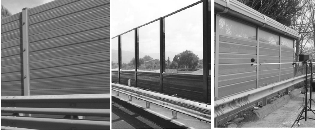
Fig. 3: the three noise barriers tested “in situ” (from left to right, sample B, C and D). On the right, 01dB Adrienne Package is shown.
