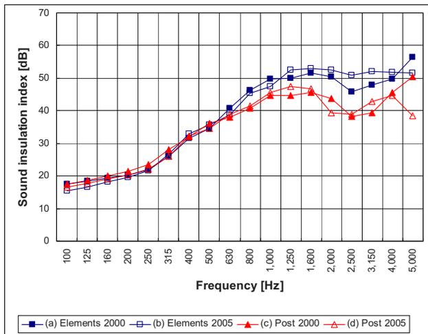
Fig. 15—Sound insulation index values measured on site B, where the metallic cassettes of a different manufacturer are installed, compared with the values obtained for the same products five years before.
