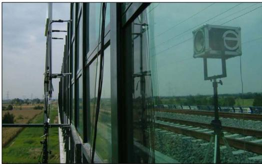
Fig. 3—Airborne sound insulation measurements: the microphone grid and the sound source in place for the acrylic barrier on the viaduct of Fig. 2.
