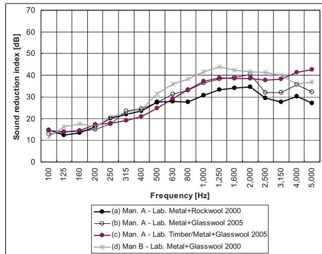
Fig. 16—Sound reduction index measured in the laboratory: (a) manufacturer A, full metal cassettes filled with rock wool; (b) manufacturer A, full metal cassettes filled with glass wool; (c) manufacturer A, timber/metal cassettes filled with glass wool; (d) manufacturer B, full metal cassettes filled with glass wool.
