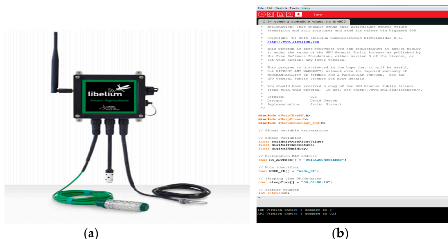
Figure 3. RSSI measurement system: (a) commercial Wireless Sensor Network (WSN) node used; (b) programming interface.
